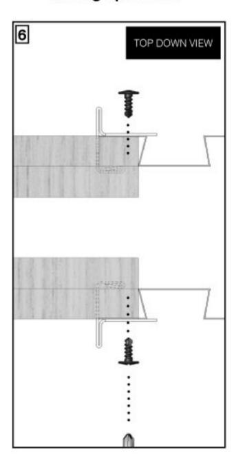
Fix the jambs onto the leading edge of the pocket. Secure with adhesive and 'Screw Set A' in top and bottom positions, and then every 400mm (pilot hole drilling not required).
