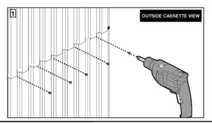
Screw through from outside to join panels together in five locations using 'Screw Set A' (pilot holes not required).
