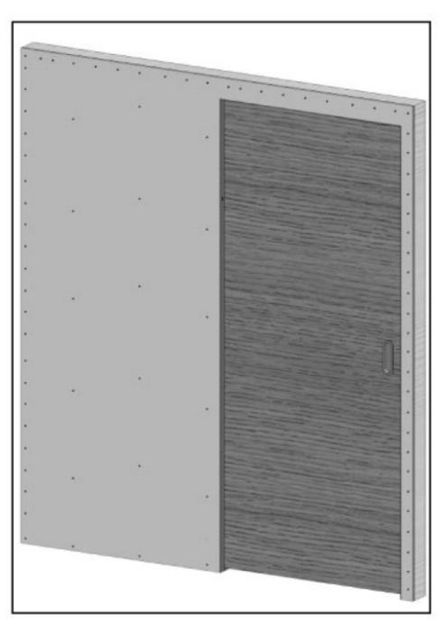
Clad the kit in 12.5mm thick plasterboard or other board material, ensuring that it finishes level and tight to the leading edge of all jambs.
