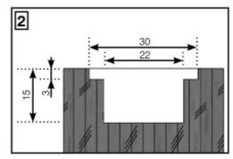
Cut the front of door mortice in the top of the door in two depth stages as pictured. Fix the cover over the mortice (screws not supplied)
