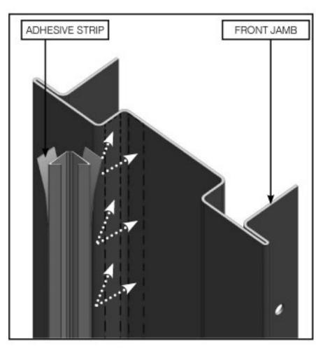
Cut the seals to the length of the front jamb. Peel back the adhesive strips and push in the two corners of the jamb.
