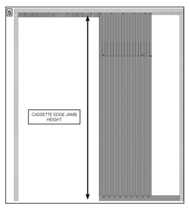
Cut the jamb to the correct height from the floor to the underside of the 'L' shaped packers.
