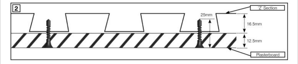
It is also required to screw fix the plasterboard to the 'Z' Section panels behind it. Ensure you
