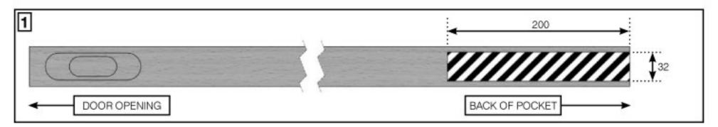
Cut the back of door mortice in the top of the door (200 x 32 x 29.5mm) and fix the bracket into this mortice (screws not supplied).
