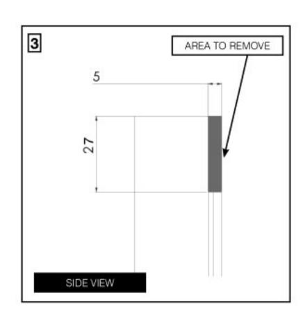
3. Make the final cut, 27mm deep, completing the cutting and removing the cut out piece.
