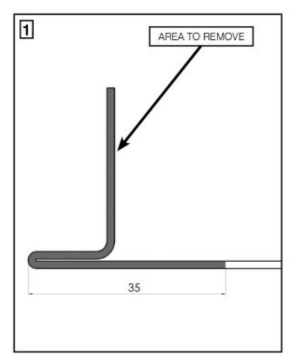
To begin, using a sawing or cutting tool, cut the head jamb 35mm from the top, cutting 35mm deep.
