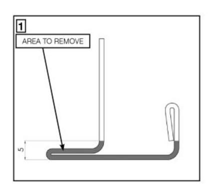
To begin, using a sawing or cutting tool, cut the cassette jamb 27mm from the top, cutting 5mm deep.
