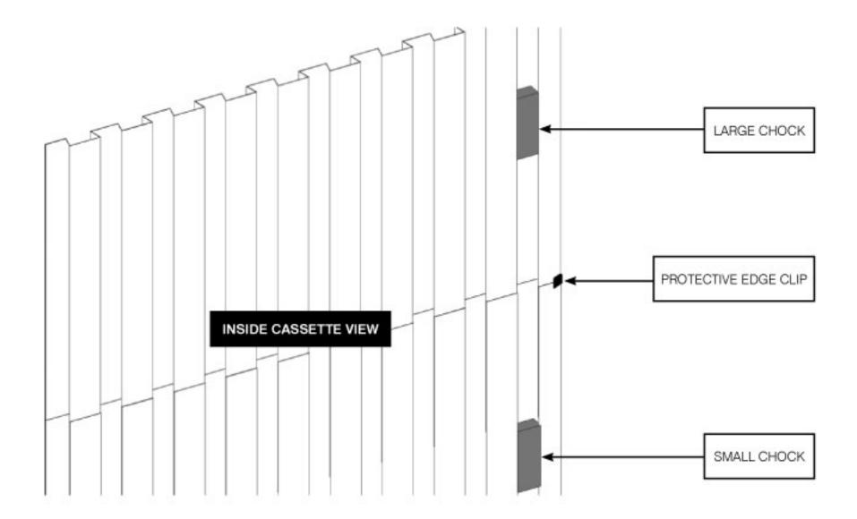
At the back of the pocket, place the protective edge clip onto the 'Z' section, covering where the panels join.
