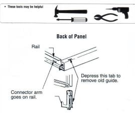
INSTALLATION HINTS: Remove door by pulling up bottom guide inserts, then lift door up and swing out. Remove guide from door frame as shown in drawing. Install new guide in same manner. Hang door and push nylon guide inserts down to engage bottom track.
