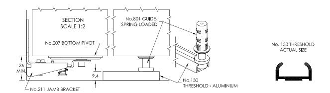
ON A CARPETED FLOOR WE RECOMMEND THE USE OF A SURFACE MOUNTED CHANNEL FITTED DIRECTLY TO THE FLOOR, WITH THE CARPET AND UNDERLAY BUTTED UP TO THE CHANNEL. A GUIDE, No. 106MF/94, IS FITTED ON EVERY SECOND LEAF DIRECTLY BELOW THE HANGER CENTRELINE.
