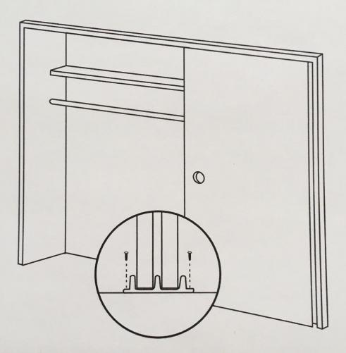
For 2-door unit, insert nylon post section in floor guide according to door thickness and locate under doors at center of opening. For 4-door unit (two guides), locate a guide 1/4" distance from each jamb, so as to engage both right and left hand pair of doors.
